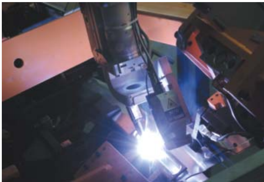
Fig. 5: Laser beam Hybrid welding at Audi: OEM in Ingolstadt applies the process for 4.5 m of weld seams in the roof area of the new A8 and thus achieves higher welding speeds and stronger seams. Photo: Audi
