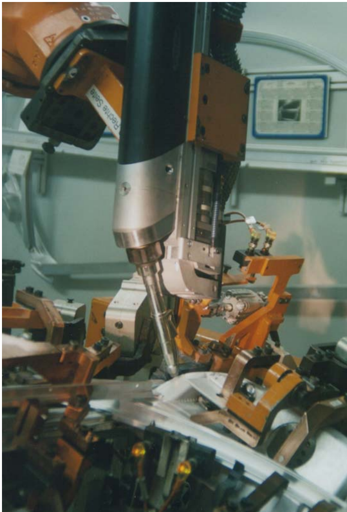
Fig. 9: The Fronius LaserHybrid welding head ensures good positionability of the laser beam and arc, both to one another and to the workpiece.
