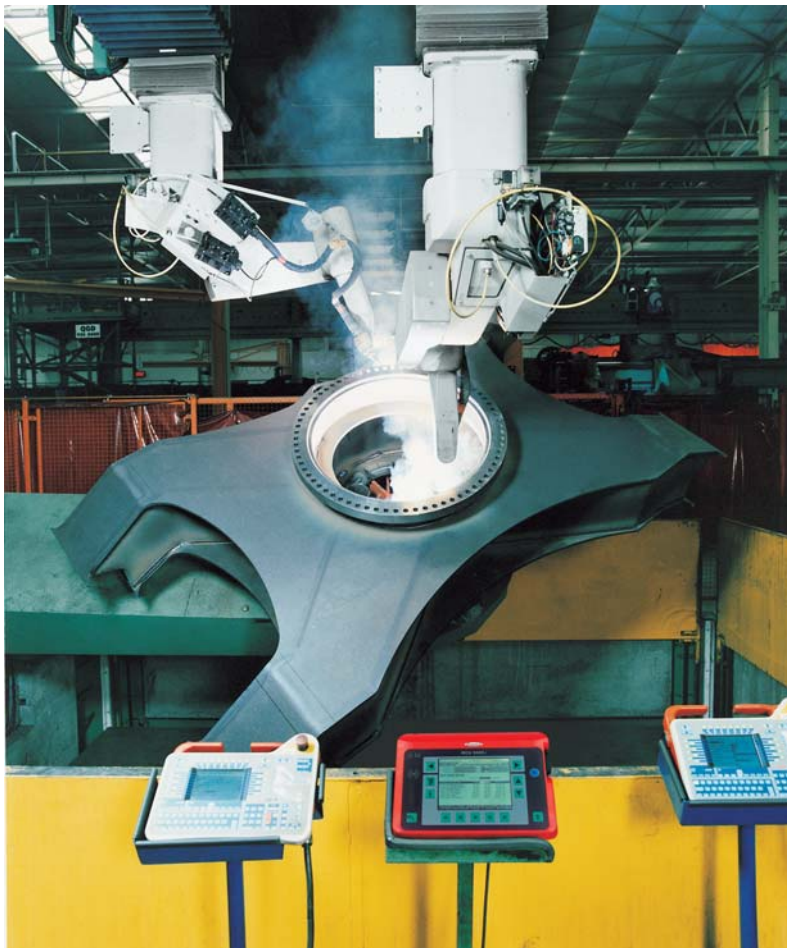
Fig. 7: Strip-wire welding is particularly suitable for joining large workpieces that can be moved by handling systems.
