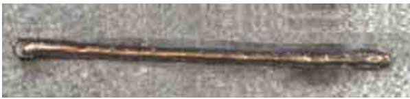
Fig. 4: Weld seam appearance where contact-tube-to-work distance was changed from 8 to 35 mm. Thanks to the exact arc-length control, virtually no spattering occurs
