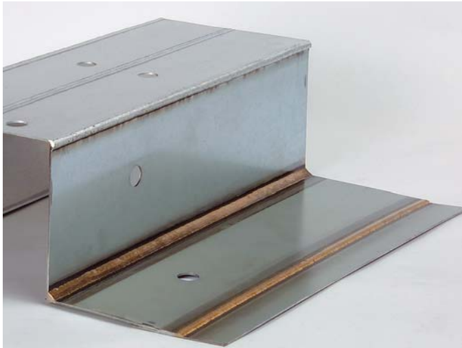
Figure 4: CMT-brazed joint between a hot-dip galvanised sheet and an electrolytically galvanised one; sheet thickness 1.0 mm, filler metal CuSi3.
