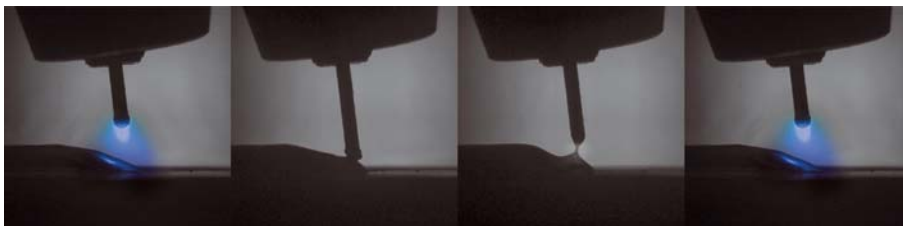
Figure 5: The principal phases in the new CMT process (from left to right): 1. During the arcing period, the filler metal is moved towards the weld-pool. 2. When the filler metal dips into the weld-pool, the arc is extinguished. The welding current is lowered. 3. The rearward movement of the wire assists droplet detachment during the short circuit. The short-circuit current is kept small. 4. The wire motion is reversed and the process begins all over again.
