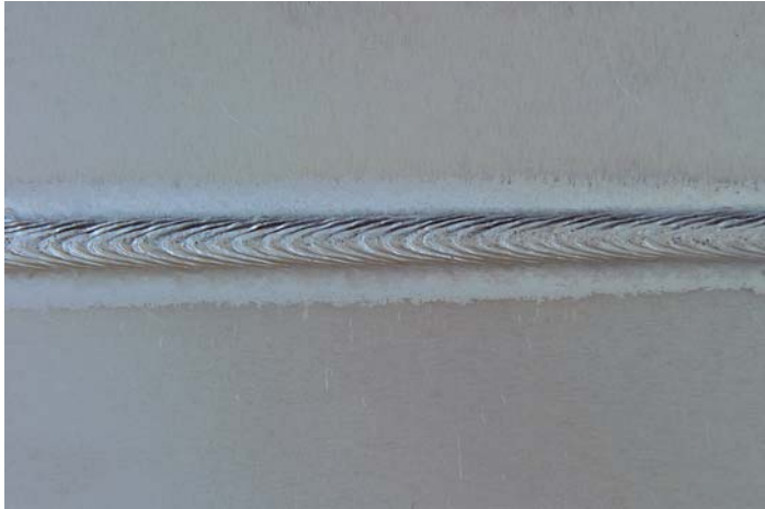
Figure 6: Fillet weld on a 1.0mm thick AlMg3 sheet, CMT-welded at a welding speed of 2.0 m/min.
