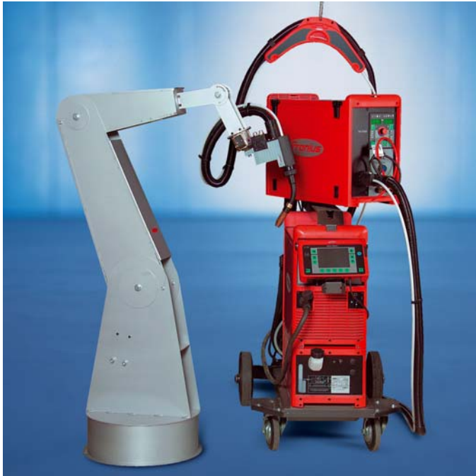
Figure 2: The CMT system - comprising the TPS 3200 CMT power source and the Robacta Drive CMT welding torch - is setting some brand-new standards in welding technology.
