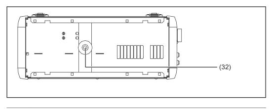
(32) Socket for swivel pin for placing the wirefeeder on the swivel pin of the swivel pin holder
