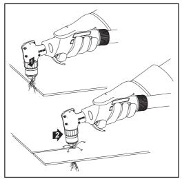
Fig. 4 Free-hand control of the cutting torch
