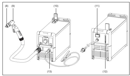
Fig.3 Connections on the front and rear of the plasma cutting device
