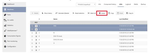
When a job was deleted, there is a progress symbol at the right hand-side showing that the delete command is progressed at the welding device. As soon as the job was really deleted at the welding device, a green checkmark appears and the job name is removed from the overview in WeldCube Premium.
