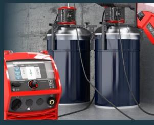
Automated switching between two wire drums
