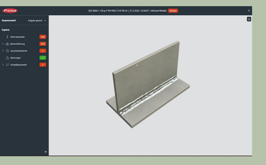
With this release, we are introducing a comprehensively revised analysis function that makes virtual welding training even more efficient. It provides a better overview of the trainee's entire task as well as detailed information such as torch guidance, exclusion criteria, welding parameters and much more. You also have the option of graphically displaying values such as angle of attack and stickout (see video)
