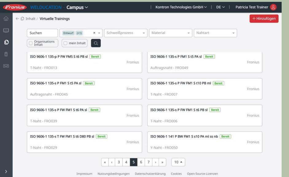
The trainer configurator can be used to create or modify virtual trainings(Welding tasks). The tool enables points such as: Adjustments of the torch, welding parameters of the welding machine, etc. and thus create additional individual training courses.
