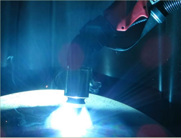
K4 fume extraction torch – extraction switched on
