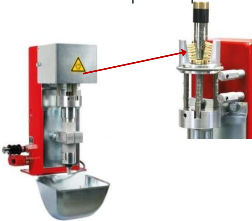
Mechanical cleaning with special brush head
