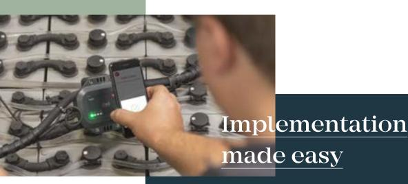
Using the NFC interface, the TagID can be configured quickly and easily via the TagID Config app. The user-friendly interface of our app assists in entering the few necessary parameters. The TagID automatically checks whether the voltage value entered during configuration matches the actual measured value. Deviations are detected immediately and consequential damage is thus effectively prevented.
