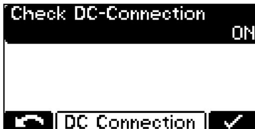
The "DC Connection" menu contains the setting for the DC connection check. If the DC connection check is switched on ("ON"), the connection between the charger and the battery is checked during the charging process.
