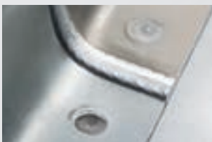
Steel - aluminium joint Material: 1) HX380 LAD+Z100, 2) EN AW-6016
