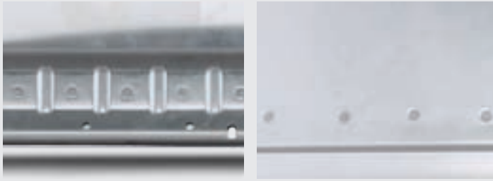
2-layer aluminium joint Material: EN AW-6016 1.3 mm
