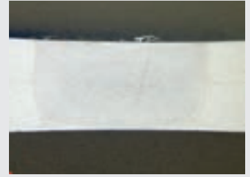
2-layer aluminium joint Material: EN AW-6016
