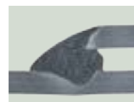
Lead: Current [A]: 280, Voltage [V]: 28.0, vs [cm/min]: 110 Trail: Current [A]: 125, Voltage [V]: 17.0, vs [cm/min]: -
