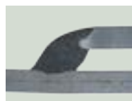
Current [A]: 155, Voltage [V]: 12.3, vs [cm/min]: 30
