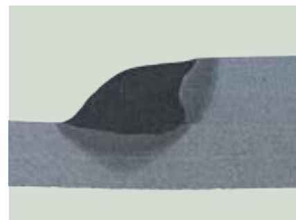
Lead: Current [A]: 440, Voltage [V]: 34.8, vs [cm/min]: 330 Trail: Current [A]: 340, Voltage [V]: 27.2, vs [cm/min]: -
