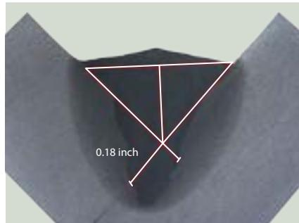
Lead: Current [A]: 440, Voltage [V]: 34.8, vs [cm/inch]: 2.75
