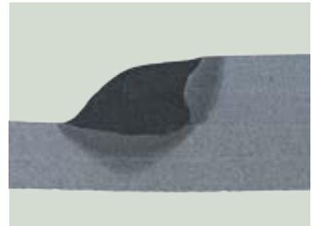
Lead: Current [A]: 440, Voltage [V]: 34.8, vs [inch/min]: 129.92
