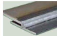
Lead: Current [A]: 280, Voltage [V]: 28.0, vs [inch/min]: 43.30
