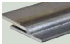
Current [A]: 155, Voltage [V]: 12.3, vs [inch/min]: 11.81
