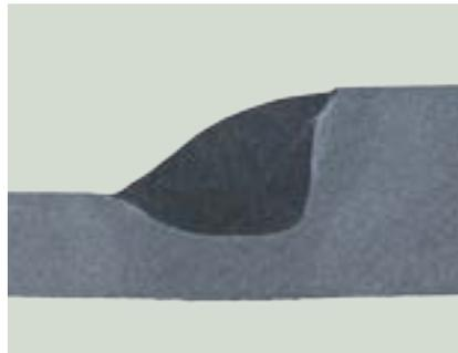
Current [A]: 406, Voltage [V]: 33.1, vs [inch/min]: 55.11
