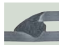
Främre: ström [A]: 280, spänning [V]: 28,0, vs [cm/min]: 110 Bakre: ström [A]: 125, spänning [V]: 17,0, vs [cm/min]: –
