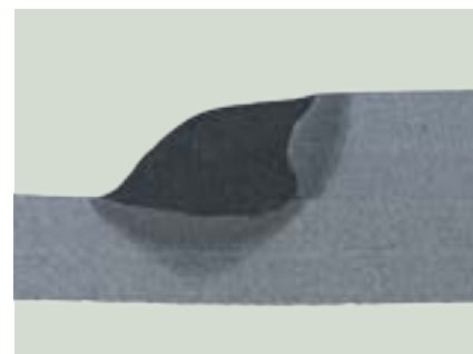
Främre: ström [A]: 440, spänning [V]: 34,8, vs [cm/min]: 330 Bakre: ström [A]: 340, spänning [V]: 27,2, vs [cm/min]: –
