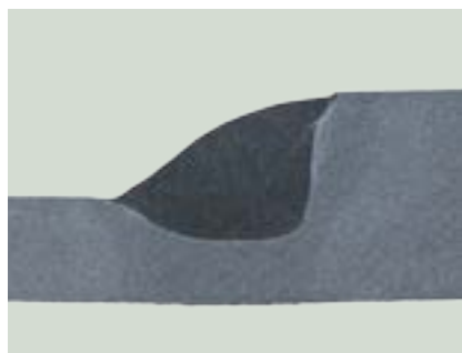
Ström [A]: 406, spänning [V]: 33,1, vs [cm/min]: 140
