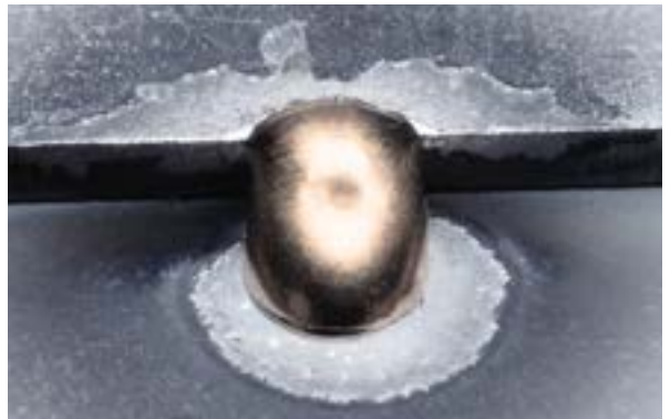
Hold point 1 mm elo coated Vd: 11,5 m/min
