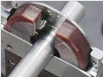
/ Excellent welding results due to closed shielding gas chamber
