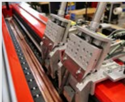
/ Adjustable pneumatic center stops
