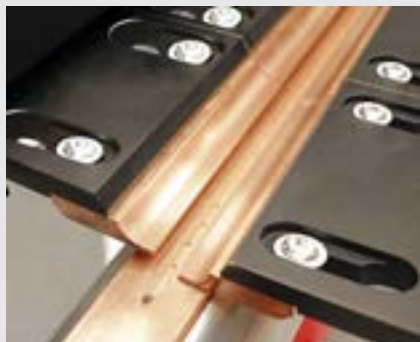
/ Backing track with forming gas holes
