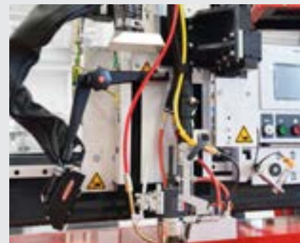
/ Weldhead with AVC/OSC slides, camera
