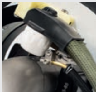
/ Wire feeding, torch bracket from 0 - 45° stepless swivelling
