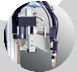
TIG weldhead with AVC slide
