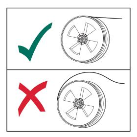
After releasing the torch trigger (end of welding, end of wirefeeding), the wirespool must stop unreeling.
