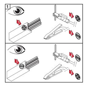
Check the rod electrode packaging to determine whether the rod electrode is for (+) or (-) welding.
