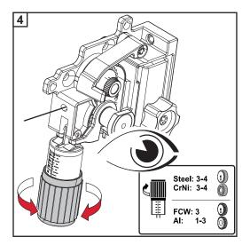
Adjust the contact pressure as shown below
