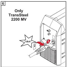
It is only necessary to connect the mains cable to the power source for multivoltage power sources.
