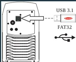
Plug in the supplied Fronius USB thumb drive with FAT32 formatting. If the power source is switched off and on again while the USB thumb drive is connected, Easy Documentation remains activated.
