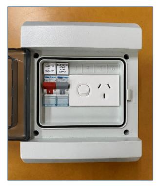
The enclosure contains an Earth bar & a Neutral bar. These are necessary to combine all the Earth connections and combine all the Neutral connections. An MEN point <u>shall NOT</u> be made within this enclosure. i.e. joining of Neutral & Earth together within the enclosure.
