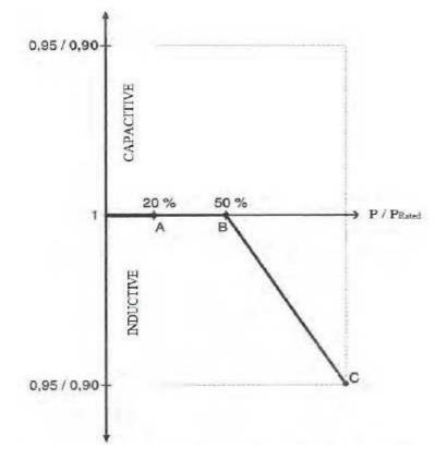
For setup BR2 / M the standard setting of point C is 0.95 (ind). For setup BR3 / L the standard setting of point C is 0.90 (ind). The curve is configurable.
