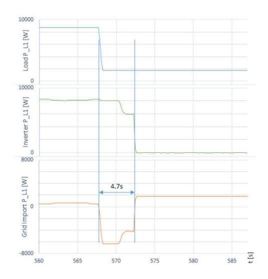
The inverter operates at a safety margin. At a change in load of 6980 W (85%) there is no export power after 4.7 s. In this case the inverter trips as a precaution at 4.7 s not to reach the 5 s limit.
