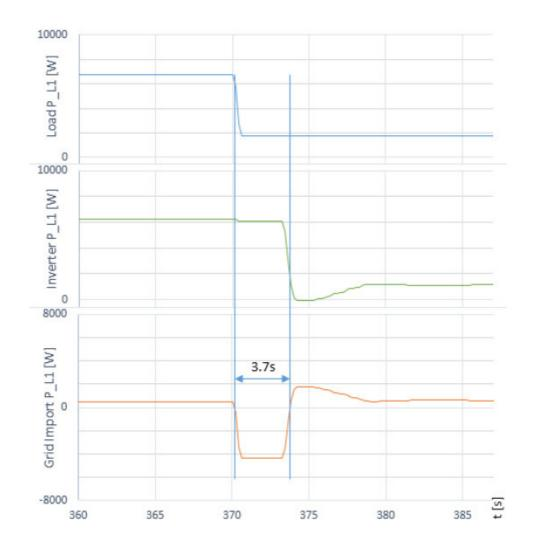
The inverter operates at a safety margin. At a change in load of 4985 W (61%) there is no export power after 3.7 s.
