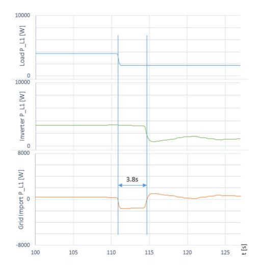
The inverter operates at a safety margin. At a change in load of 1970 W (24%) there is no export power after 3.8 s.
