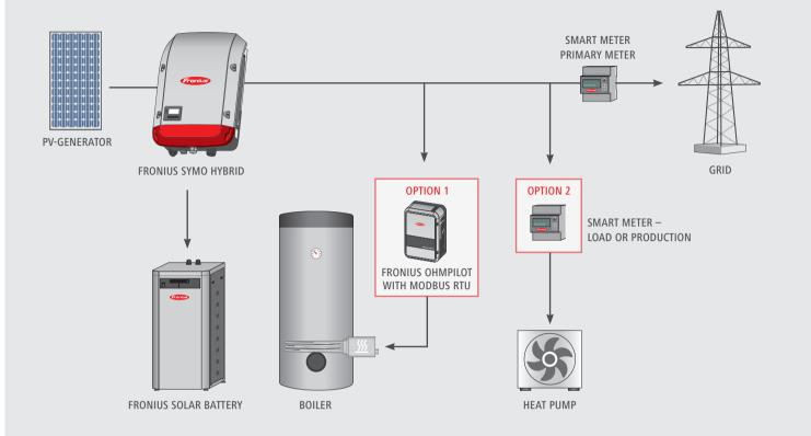
Option 1: Ohmpilot connected via Modbus RTU with one Fronius Smart Meter (primary meter)
