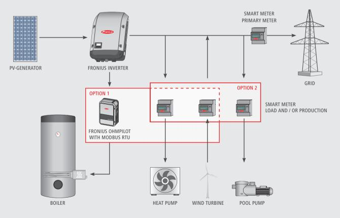
**Option 1:** Ohmpilot connected via Modbus RTU with **three Fronius Smart Meters** (one of which is the primary meter) **Option 2:** Without Ohmpilot (or Ohmpilot connected via TCP/Wlan) with **four Fronius Smart Meters** (one of which is the primary meter)
