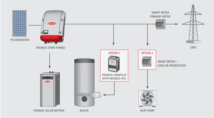
Option 1: Ohmpilot connected via Modbus RTU with one Fronius Smart Meter (primary meter) Option 2: Without Ohmpilot (or Ohmpilot connected via TCP/Wlan) with two Fronius Smart Meters (one of which is the primary meter)
