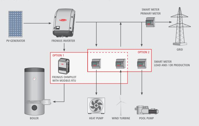
Option 1: Ohmpilot connected via Modbus RTU with three Fronius Smart Meters (one of which is the primary meter)
