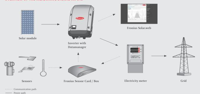
The Fronius Sensor Card / Box offers inputs for up to six measuring signals.
