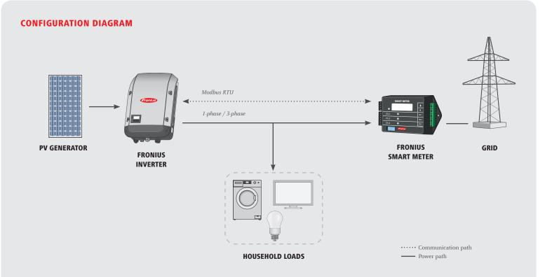
The Fronius Smart Meter is compatible with all inverters with an RS485 interface (Modbus RTU). The Fronius Smart Meter works in conjunction with the Fronius Datamanager 2.0 for the Fronius IG Plus inverters. The Fronius Smart Meter can be retrofitted at any time together with the Fronius Datamanager 2.0 in inverters that have already been installed.
