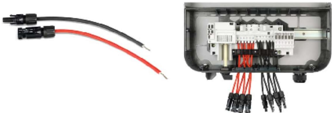
/ The MC4 cable option enables inverters to be cabled-up quickly and easily, which in turn allows a rapid PV system connection process. The option can be ordered on an individual basis per string (2 to 6 strings) and has been specially designed for use with Fronius Symo 10.0 – 20.0 kW and Fronius Eco inverters. The inverters are delivered with the installed MC4 cable option<sup>1)</sup>.
