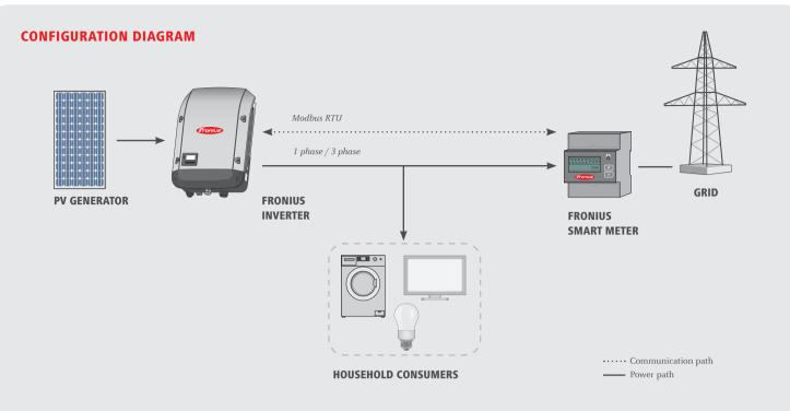
/ Function supported by all Fronius SnapINverter inverters with integrated Fronius Datamanager 2.0, Fronius Smart Meter is required. Fronius Datamanager 2.0 and the Fronius Smart Meter can be retrofitted at any time into pre-installed inverters.
