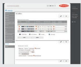
/ Dynamic power regulation takes into account the current energy requirement in the household before implementing a PV system power reduction. For this, Fronius inverters can be easily connected to a Fronius Smart Meter via the Modbus RTU interface. The bidirectional meter records and optimises selfconsumption and offers extremely rapid and precise dynamic feed-in management. Together with Fronius Solar.web, the Fronius Smart Meter provides a transparent overview of energy usage within the home.
