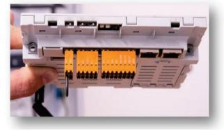
Figure 6.2.2.b: GEN24 Pilot connection area
