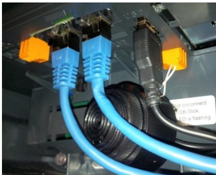
Figure 7. Buzzer connection with Signal relay and 5V USB power supply
