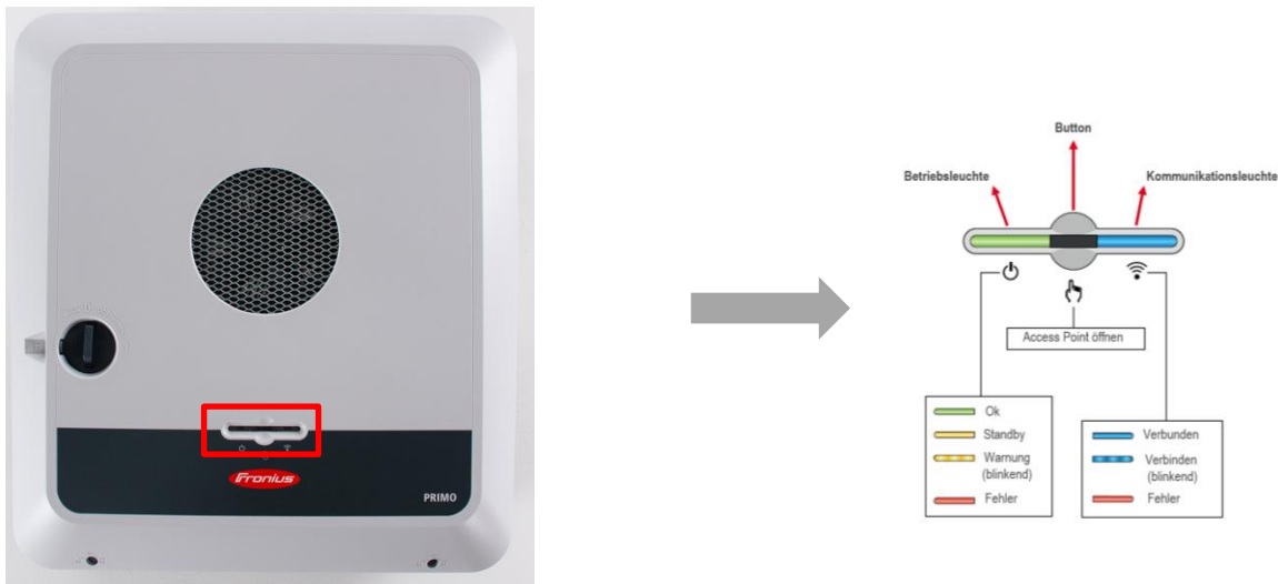
Figure 9: Opening the local network (Wifi access point) of the Fronius GEN24 inverter series and description of the functions of the LED patterns.
