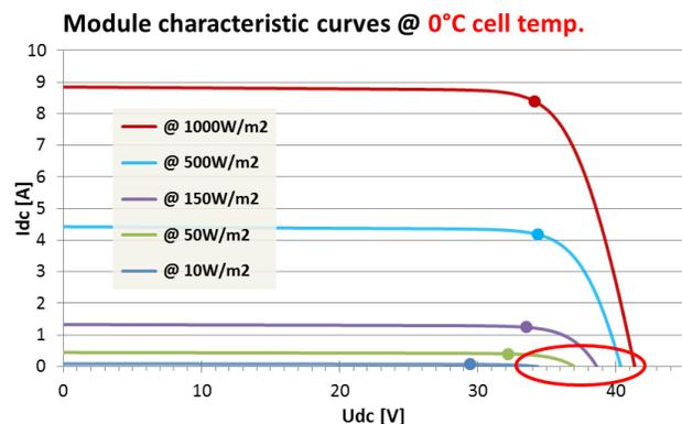
Figure 2: irradiation dependency of the open circuit voltage @ constant cell temperature (0°C)
