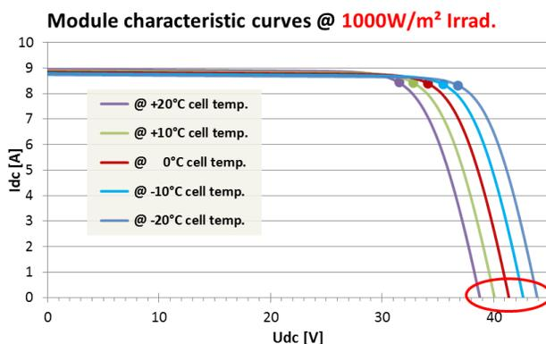
Figure 1: temperature dependency of the open circuit voltage @ constant irradiation (1000W/m<sup>2</sup>)
