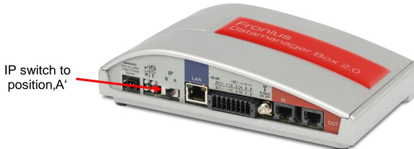
Figure 3: Fronius Datamanager 2.0 Box connection area
